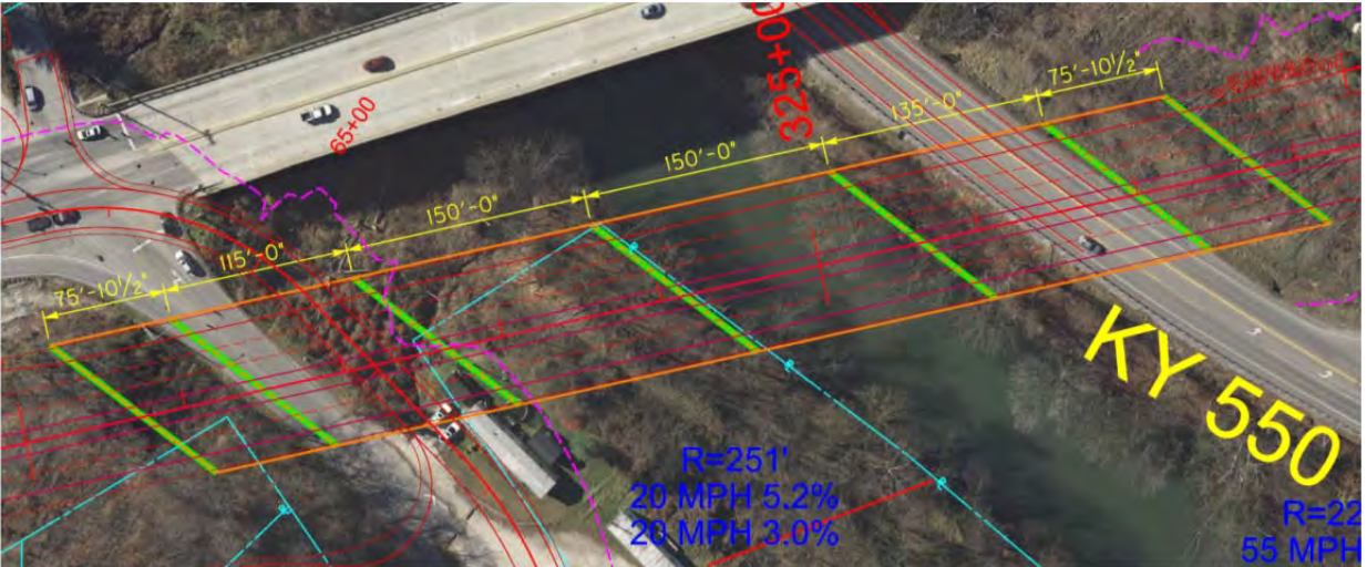
Figure 9 - VE Team recommended span lengths
